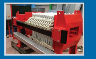
Filter Presses are dewatering equipments with the highest dewatering rate among all the mechanic dewatering equipments used. By transforming sludge like solid material into cake, the filter press separates water. Moreover, this kind of press is the most widely used dewatering system due to its economical and ease of use qualities.
